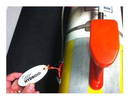
**Magnet** (with floating keychain) is installed beside the orange Iridium/GPS antenna to shut the vehicle OFF.
