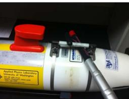
AUV showing forward and aft **handles** that can be used for handling/lifting the vehicle by hand and catching the vehicle with a pole for recovery. Anything orange is delicate and cannot be grabbed by hand. The AUV will be deployed and recovered from a swimstep or side of small boat.
