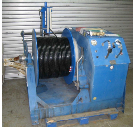
Winch and E-M cable
