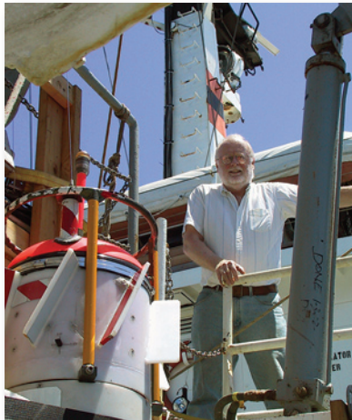
Tom at sea with the Absolute Velocity Profiler, his ocean density and velocity profiler based on e-field sensing.
